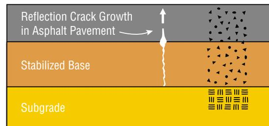
Care must be taken in determining what mechanism is causing cracks in the asphalt surface. They can occur for a number of reasons, such as poor construction, structural failure, asphalt aging, temperature cracking, etc. The only way to be sure a crack in the surface of an asphalt pavement is reflecting a crack in the stabilized base layer is to take a pavement core and visually see the crack in the same location in the base and asphalt layers.
