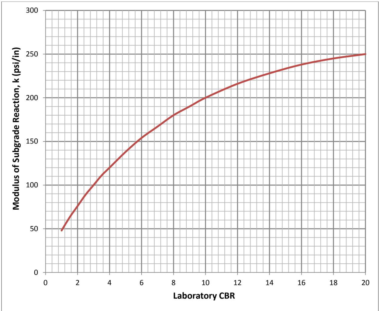
Figure 1. Relationship between laboratory CBR and k value.
