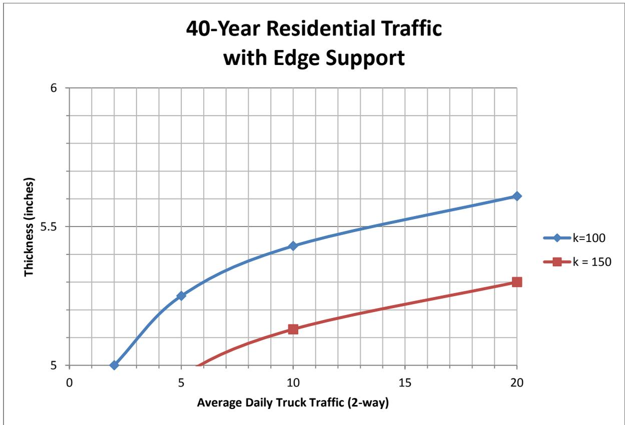
Figure 7. Design Chart A. (For k greater than 150, use 5 inches.)
