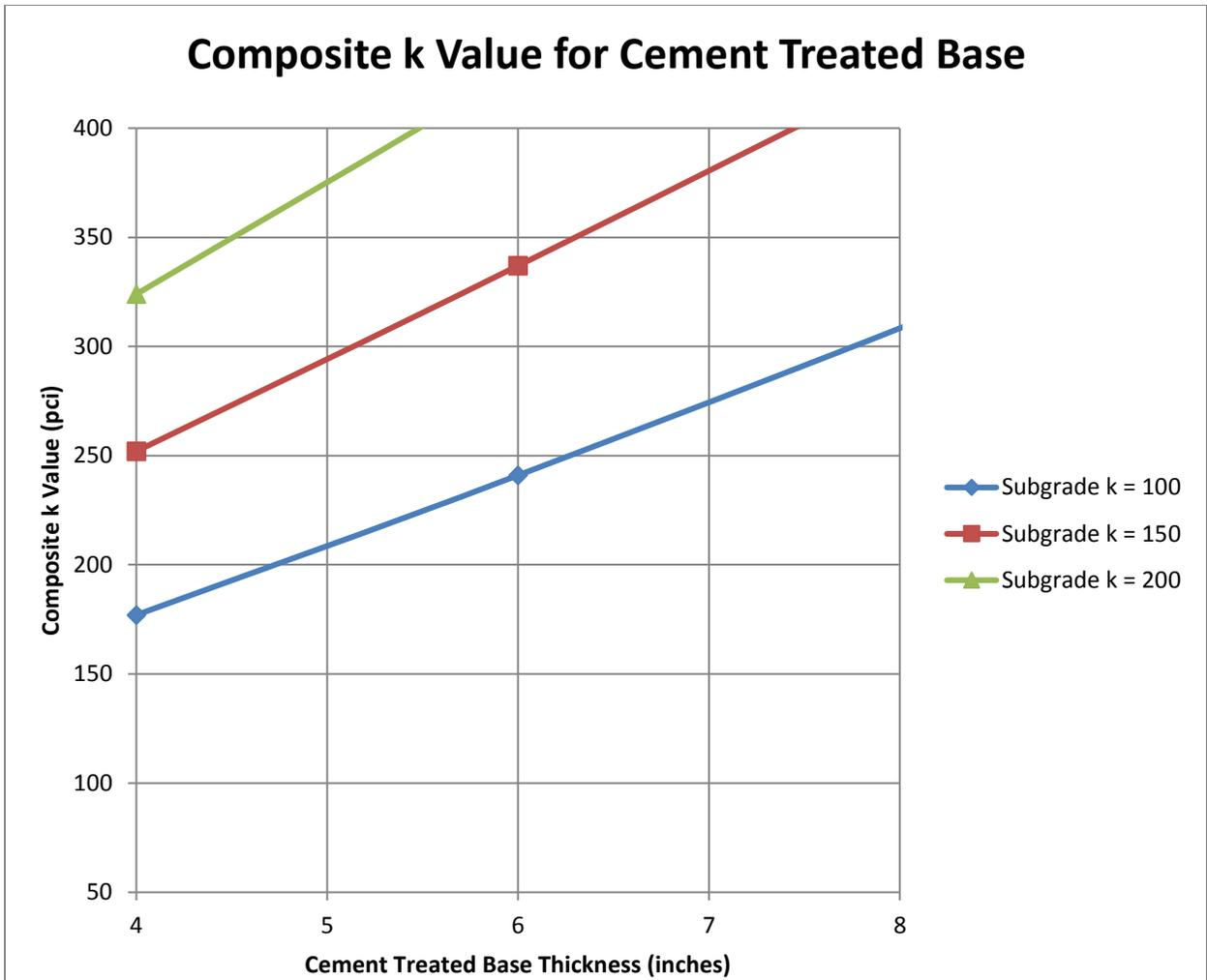
Figure 3. Composite k Value for Cement Treated Base.
