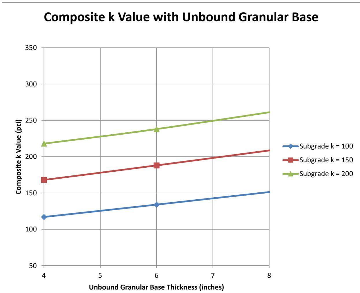
Figure 2. Composite k Value for Unbound Aggregate Base.
